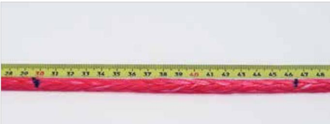
Mark the rope in locations 30 cm and 46 cm from the tip (with an eye size of 5 cm).
