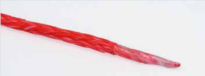
Form the rope end into a tip and wind adhesive tape around it.
