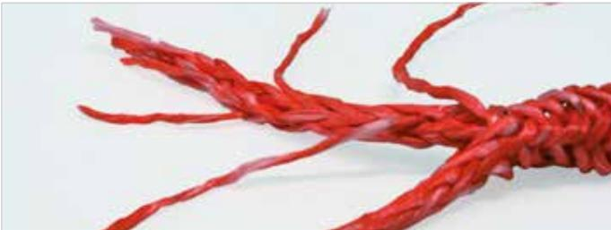
Remove the adhesive tape and taper the rope's end such that 30% to 50% of the strands are extracted from the rope's end at equal distances and severed.
