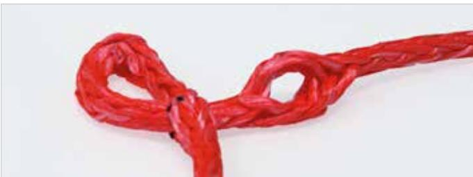
Open the tipped rope end after 2 plaits (2 - 3 cm) again in the center (equal number of strands on both sides). This is the second opening.
