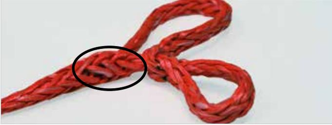
Insert the tipped end into the rope.
