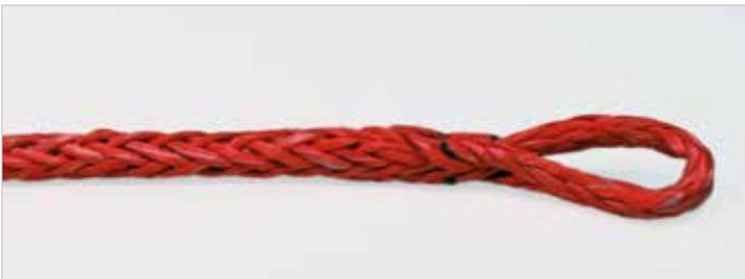
Smooth out the splice such that the tapered rope end disappears inside the rope.
